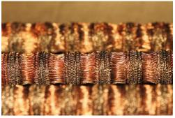
For efficient evaporation of the natural refrigerant water, it is necessary that the heat exchanger has a large specific surface area, as shown by this sheath structure of woven and knitted copper wire soldered to the round copper pipe. ©Fraunhofer ISE
