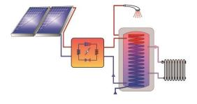
Schematic of a combined heat pump and PVT collector system for supply space heating and hot water heating. ©Fraunhofer ISE
