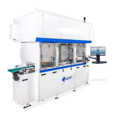
The SST 8301 Automated Vacuum Soldering System placed at Fraunhofer IISB.
