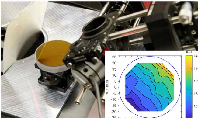
Measurement setup and result for film thicknesses of a concave mirror.
