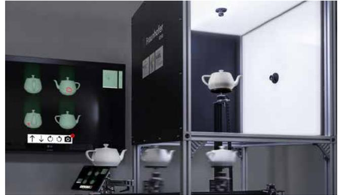
*Integrated cameras in our Halodome system detect any anomalies on products like this tea pot, our demonstration object.*
