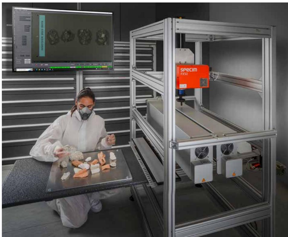
*State-of-the-art camera technology is used to acquire image data in the hyperspectral imaging lab for training AI models.*
