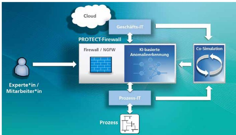
*Basic concept of agent-based network simulation and transparent attack detection.*
