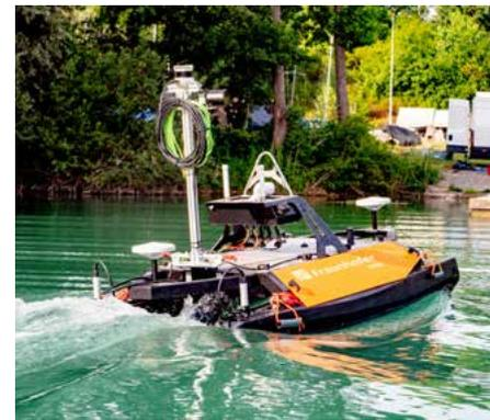
TAPS — autonomous sensor carrier.
