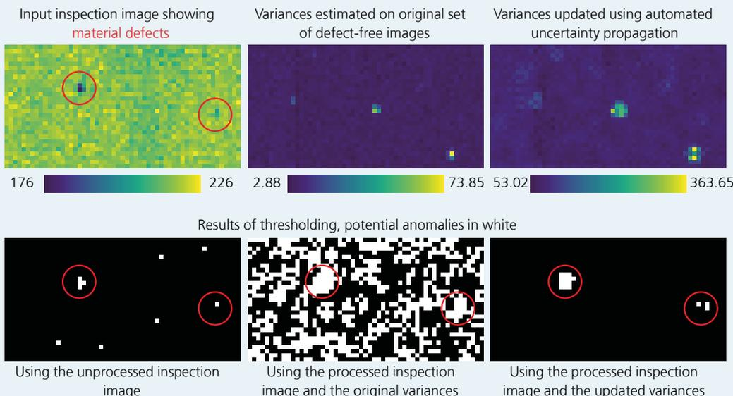
Experimental results of the implemented anomaly detection framework: Without using AutoUncertainty to calculate the correct pixel-wise statistics, several false events would have been detected (lower left image). The correct statistics allowed to only detect the actual material defects (lower right image).
