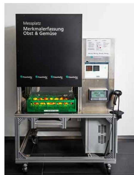
*The AI-based analysis of standard fruit crates is performed directly on the multisensory scanner.*
