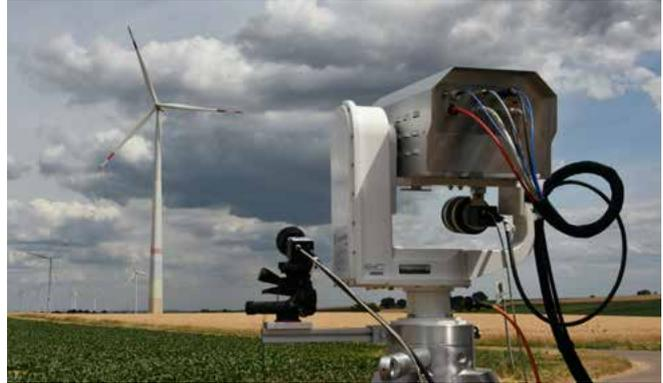
*Laser Doppler vibrometer for taking measurements on moving objects.*
