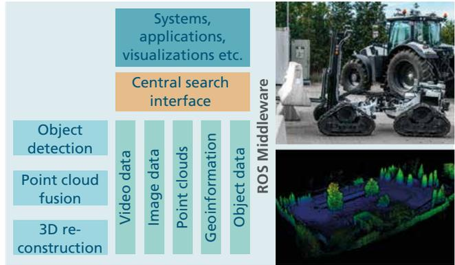
Overview of the components of the MUSAL ecosystem, sample autonomous mobile systems, and generated point cloud data.
