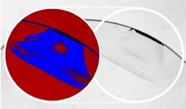
*The advantage of light field illumination (left) in direct comparison to traditional bright field illumination of the same specimen.*
