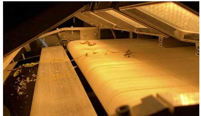
Fast-switching pneumatic valves remove plant particles contaminated with PAs.
