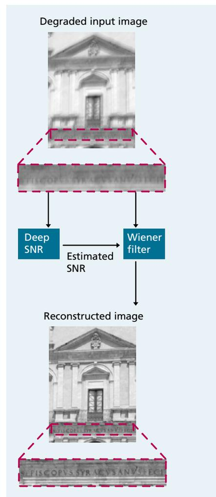
Example application of DeepSNR-based Wiener filtering of a degraded input image from [2].
