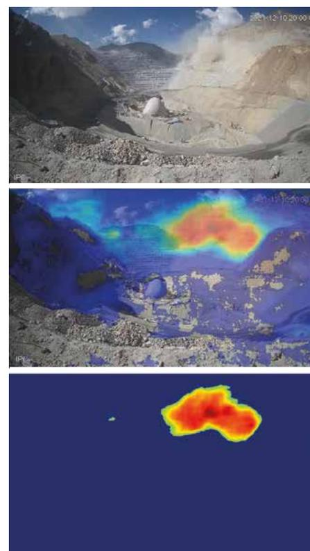
Open-pit copper mine in the Chilean highlands with dust cloud detection result. The opacity estimate is color-coded or displayed in 3D as elevation.
