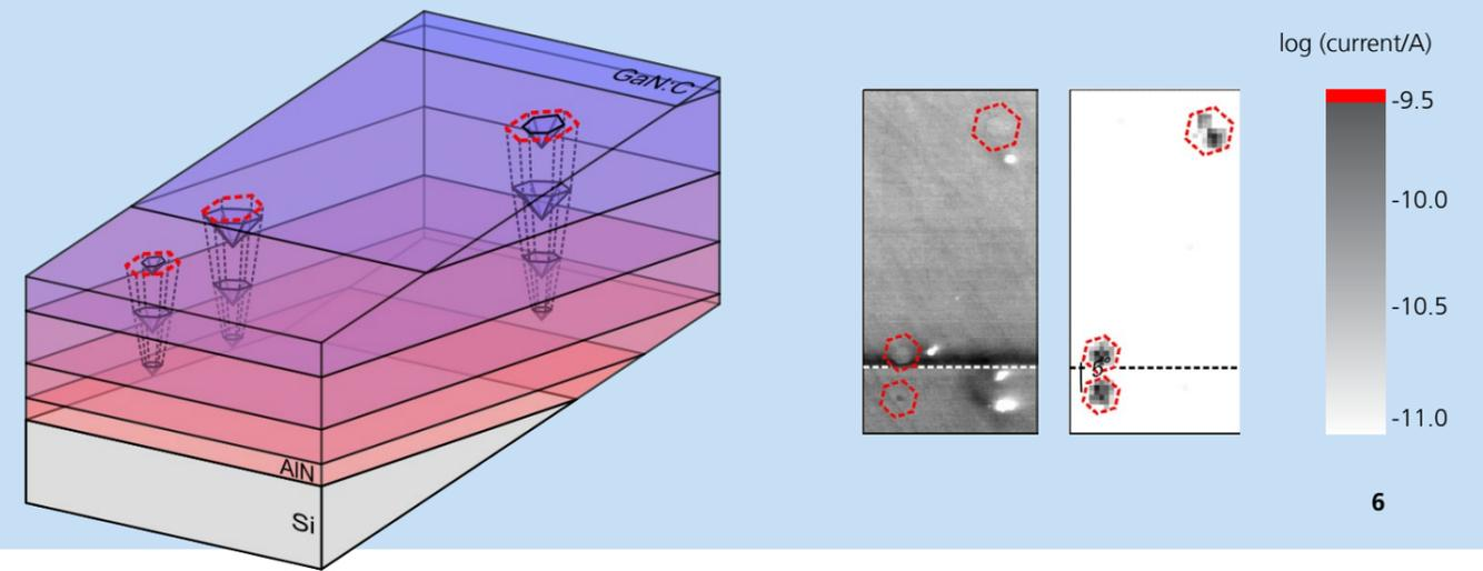
Moreover, the study showed a vertical breakdown limitation of typical GaN on Si HEMT structures due to other defects like dislocations by extrapolating the found relationship to zero V-pits below the device.
