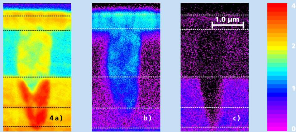
Different samples have been investigated with regard to the presence of V-pits in the multi-layer structure by cross-sectioning and the fabrication of slanted samples. It turned out that not only the presence of V-pits within the nucleation layer itself, but also the efficiency of over-growth in the layers above is strongly dependent on nucleation layer growth conditions (see Fig. 5).
