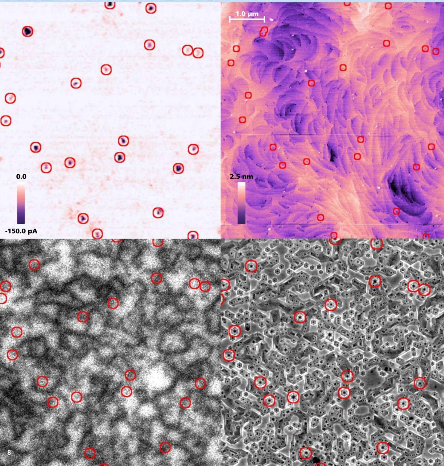
A direct correlation to the sample topography measured by AFM, the full underlying dislocation structure measured by Cathodoluminescence and the etch pit distribution and geometry after defect selective etching showed that first only a portion of dislocations is able to conduct current within the detection limit of the setup and second that only dislocations with screw component are candidates for that, but never dislocations of pure edge type (see Fig. 8).
