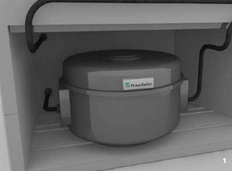
1 + 2 CAD model of a magnetocaloric cooling system. A rotating permanent magnet generates a magnetic field that heats and cools the series-connected magnetocaloric segments.
