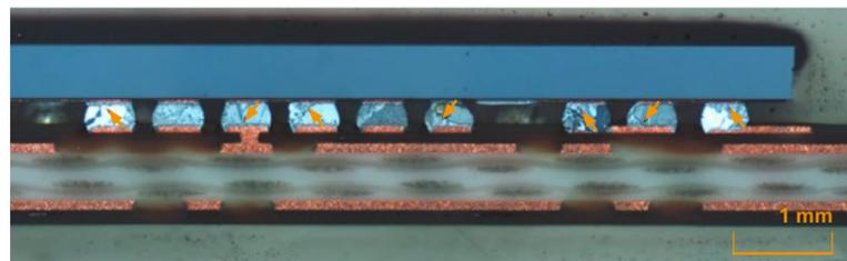
Figure 7b: Dissolution of the chip metallization
