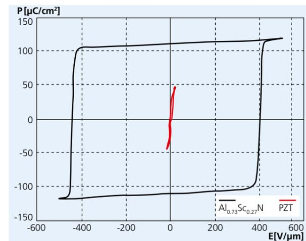
Figure 2: Ferroelectric hysteresis loop of AlScN compared to PZT – considering the key ferroelectric properties such as the remnant polarization, AlScN offers unmatched performance
