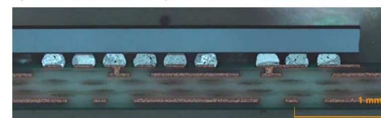
Figure 6b: Thick phase solder
