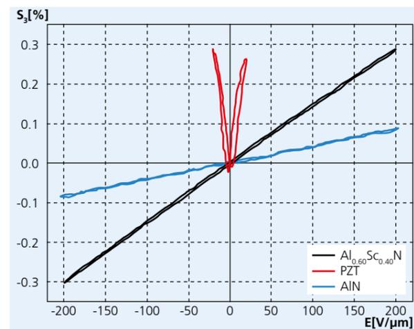
Figure 1: Comparison of the piezoelectric displacement in PZT, AlN and AlScN. Due to large coefficients and superior stability, AlScN offers excellent strain and linearity at the same time
