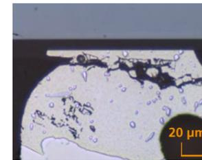
Figure 9: Strong phase growth without dissolving the chip metallization
