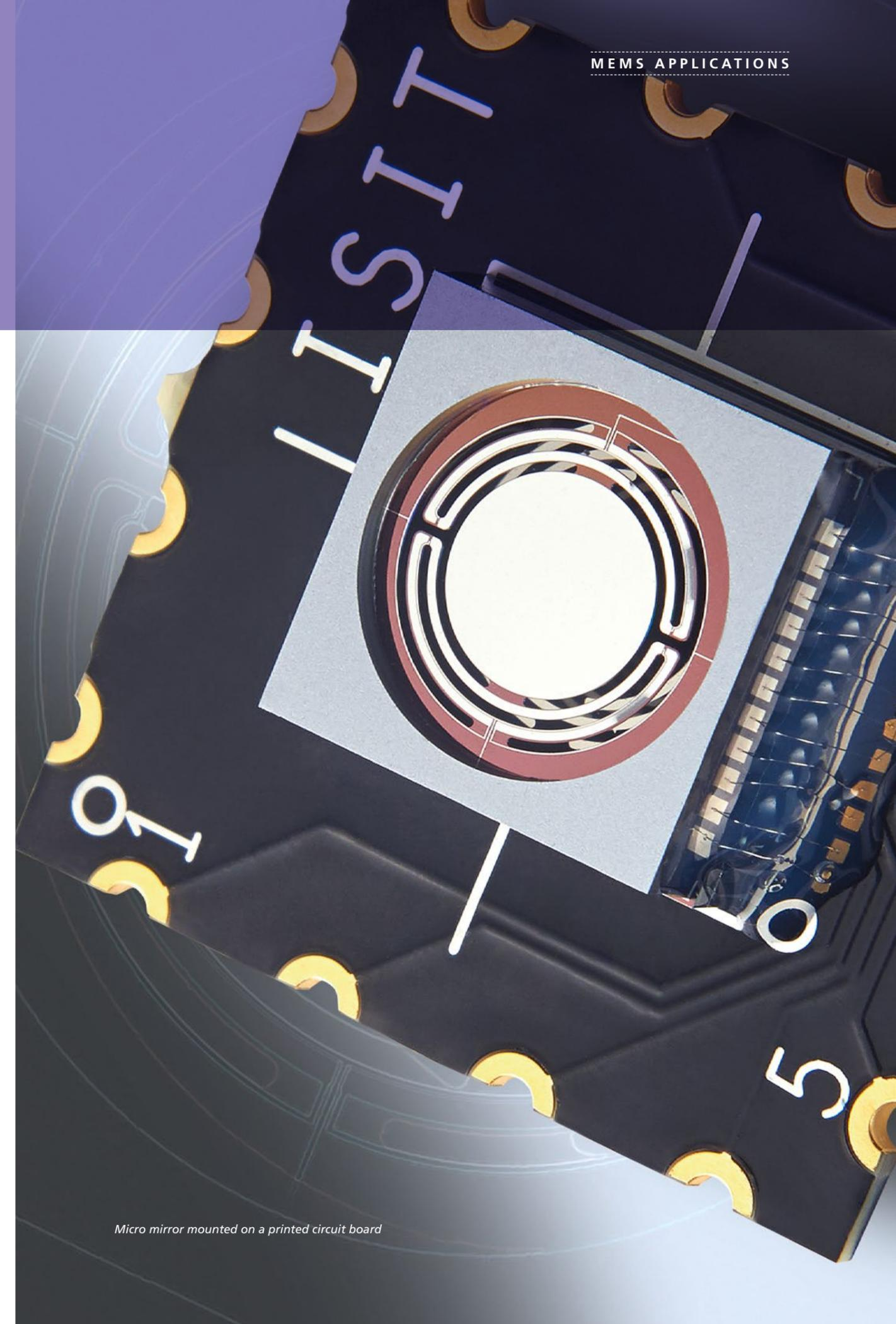
Micro mirror mounted on a printed circuit board
