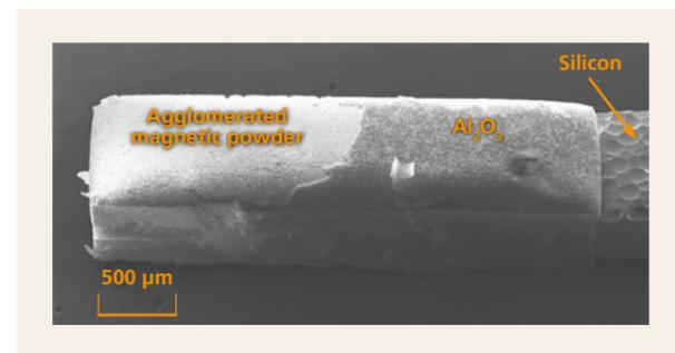
Figure 2: SEM image of the core P04, after partly removal of the surrounding silicon by etching in XeF<sub>2</sub> gas phase
