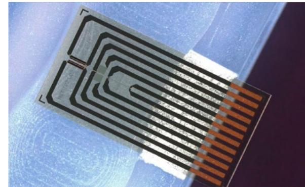
Glass chip with sensor elements to measure water flow, conductivity and temperature
