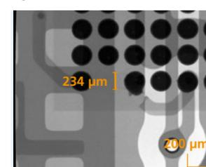
Figure 4: Molten solder ball
