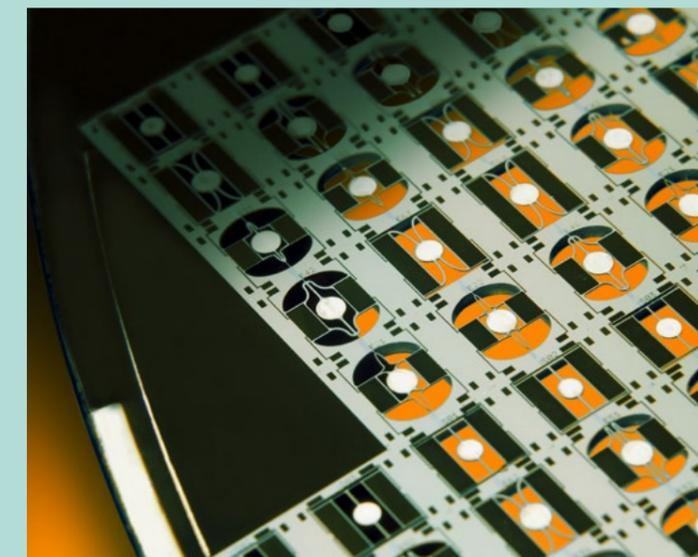
Scanning micro mirrors with experimental suspensions
