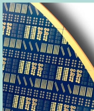
Left: GaN on Si wafer with test structures for measurement of n-type and p-type contact
