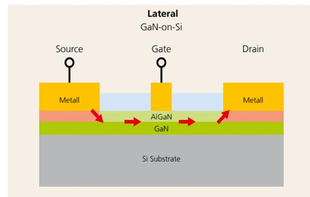
Figure 1a: Schematic of a lateral GaN HEMT device; red arrows show the current path
