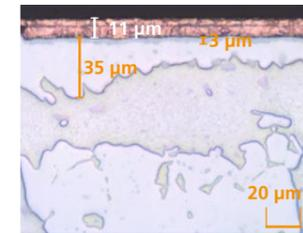
Figure 10: Complete dissolution of the PCB metallization
