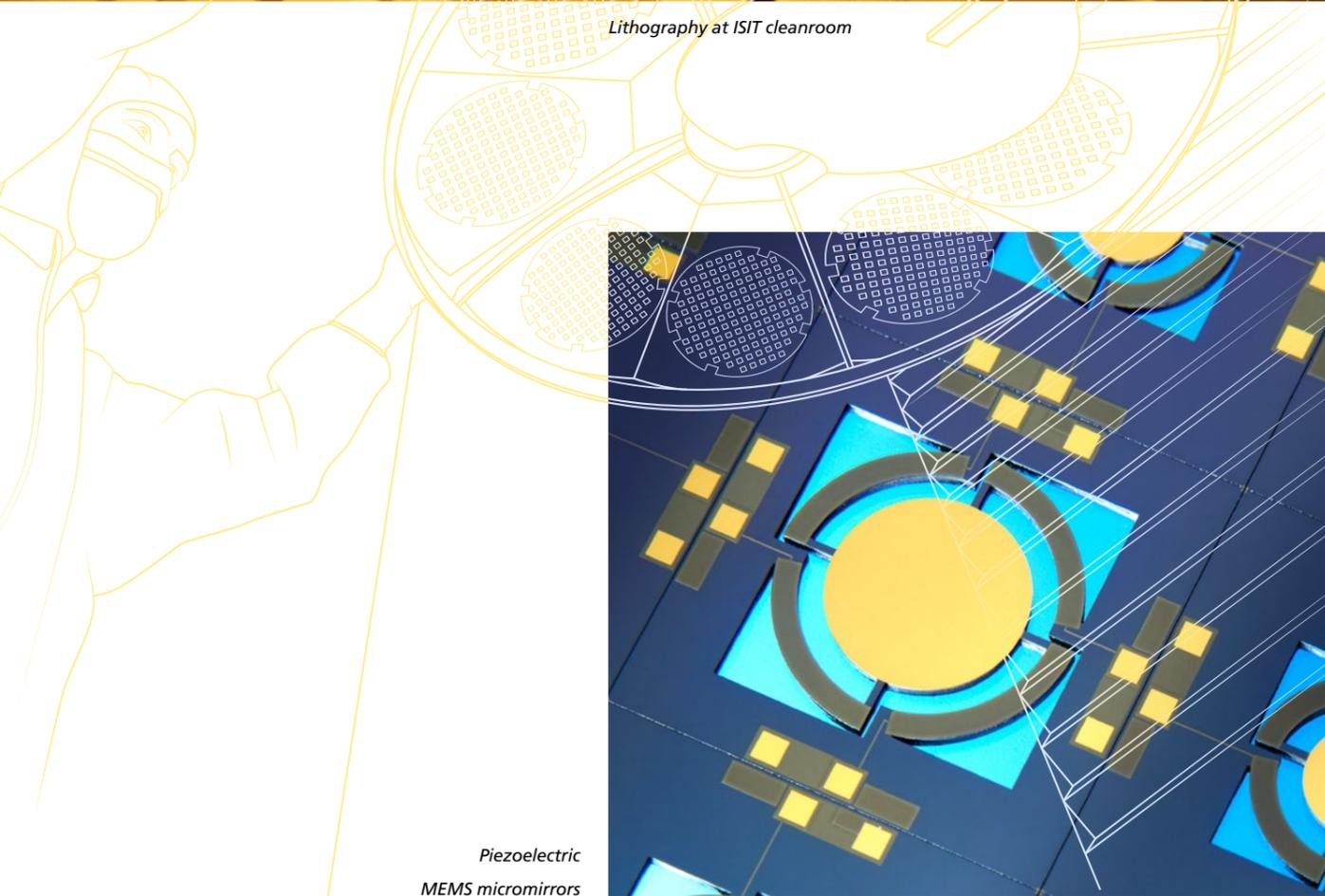
Piezoelectric MEMS micromirrors
