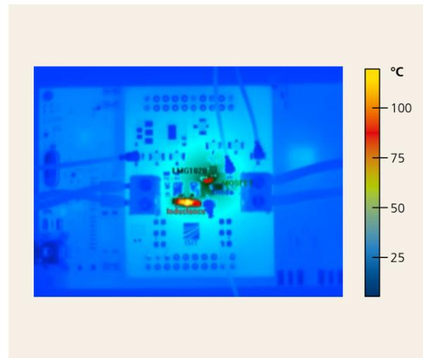
Figure 6: Thermal image of the boost converter
