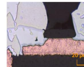
Figure 12: Phase growth without current and temperature load
