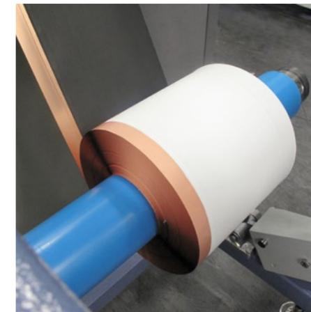
Figure 2: Electrode (anode) coated with separator at Fraunhofer ISIT
