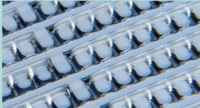
Above: Fabrication of packages for laser diodes
