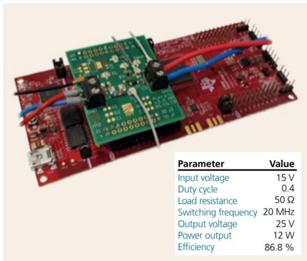
Figure 5: Boost converter prototype with inductor test sample P 04
