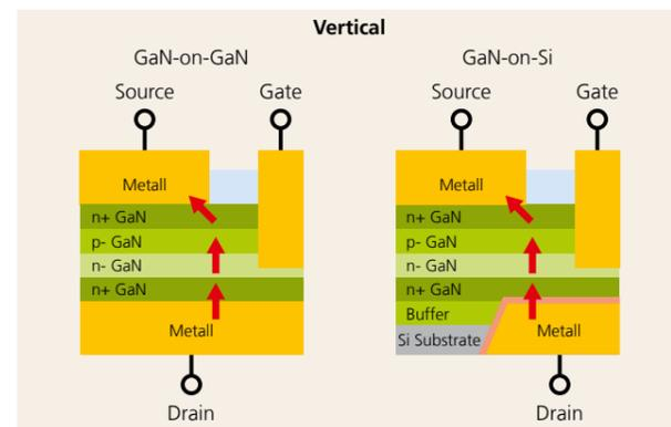
Figure 1b: Schematic of vertical GaN devices; red arrows show the current path
