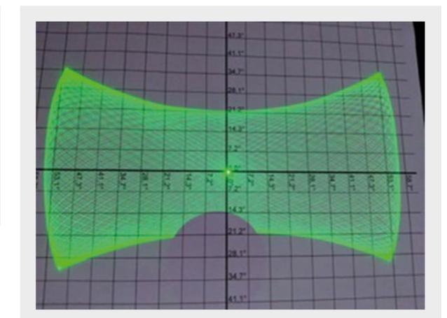
Figure 3: Result of biaxial scanning angles driven by  $\pm 40$  V<sub>AC</sub> at  $f_x = 2.26$  kHz and  $f_y = 2.3$  kHz, respectively. The maximum total optical scanning angles are  $\vartheta_{opt,x} = 55^\circ$  and  $\vartheta_{opt,y} = 35^\circ$ , where a distortion less rectangular field of view has an area of  $50^\circ \times 20^\circ$
