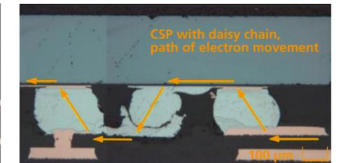
side (UBM, Under Bump Metallization) and on the PCB side goes into solution, which has two effects: The more copper is consumed, the stronger the phase growth. But as the copper becomes thinner, the temperature in the solder gets higher until it is partially melted. The phase growth is strongest on the PCB side. Figures 8 to 13 show detailed images of the solder joints.
