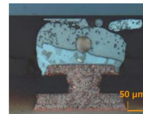
Figure 11: Partial dissolution of the PCB metallization
