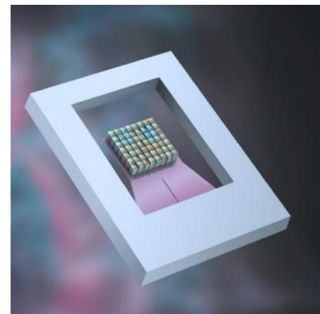
Magneto-sensitive piezoelectric energy harvester
