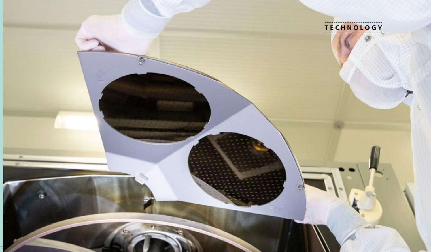
Operator loading wafers into the evaporation chamber
