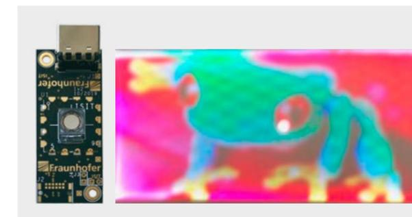
Figure 2: Left: Vacuum packaged MEMS mirror mounted on a PCB for closed-loop driving. Right: Laser projection picture based on Lissajous scanning using double resonant axes
