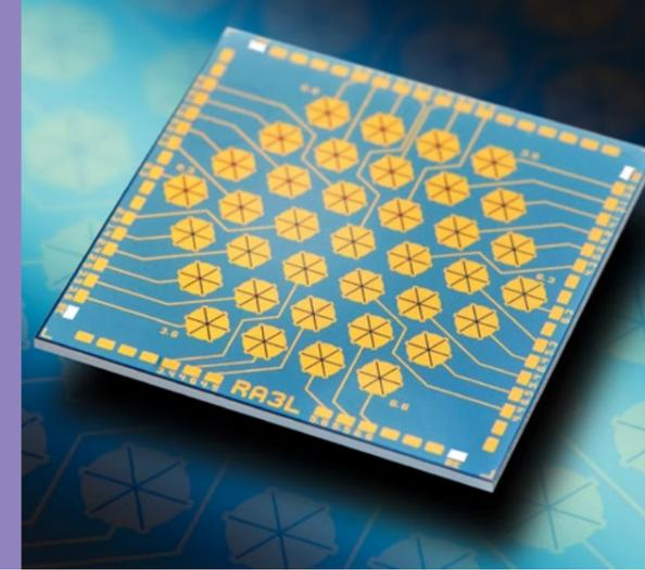
MEMS chip with piezoelectric ultrasound transducers
