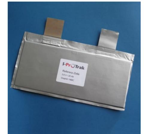
Figure 3: 20 Ah prototype cell with directly coated separator
