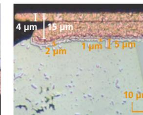
Figure 13: Phase growth with temperature load without current
