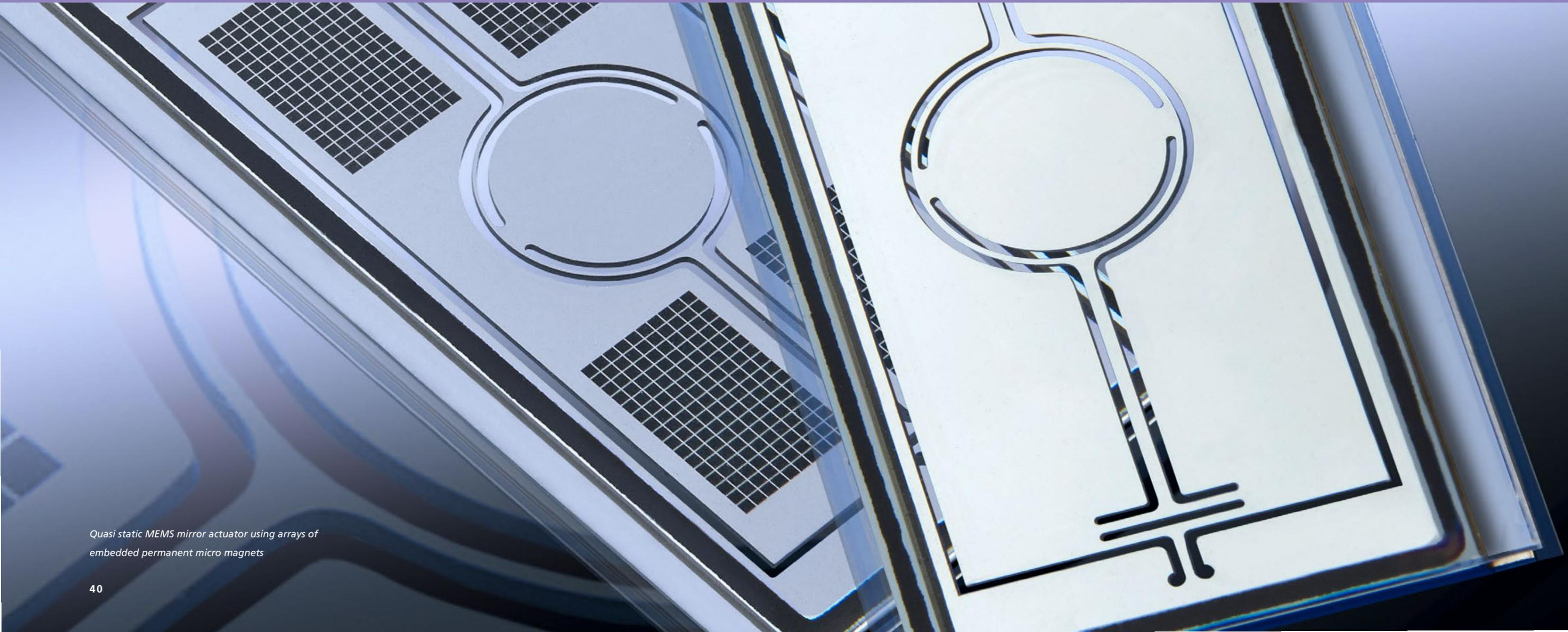
*Quasi static MEMS mirror actuator using arrays of embedded permanent micro magnets*
