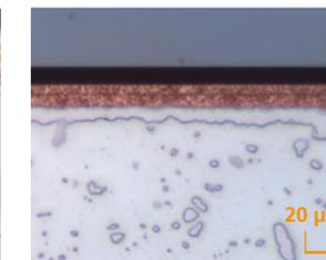
Figure 8: Complete dissolution of the chip metallization
