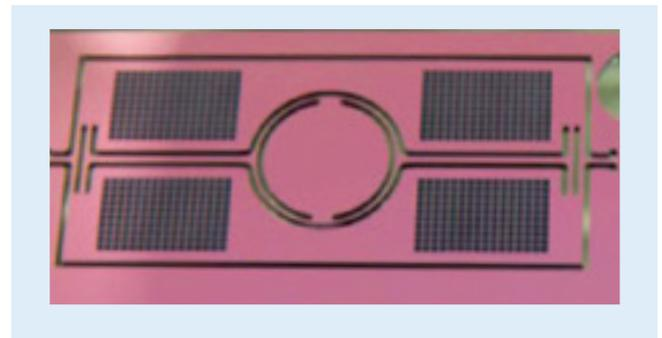
*Figure 4: Quasi-static MEMS mirror actuator using four arrays of embedded permanent micro-magnets*
