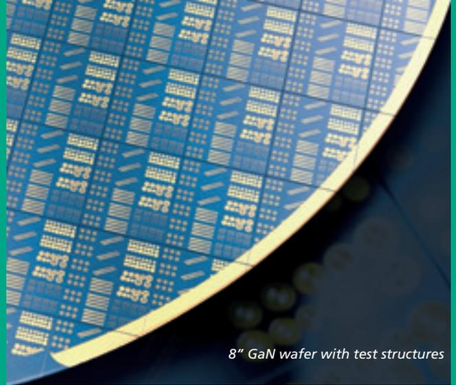
*8" GaN wafer with test structures*
