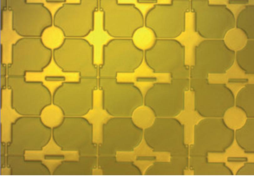
Figure 2: Microscope image of the piezoelectric actuator layer
