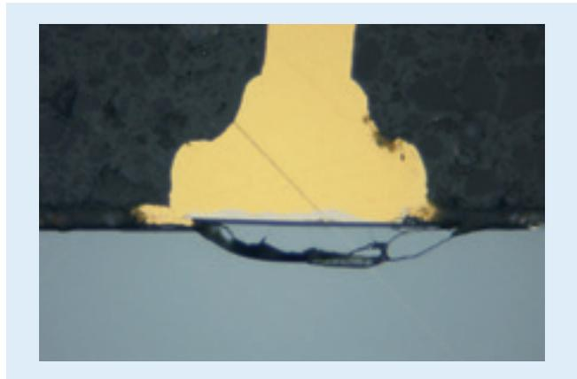
Figure 5: Crack in surface Si below a wire bond contact
