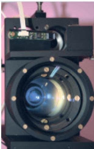
*Figure 2: Example of a 2D MEMS scanner design*
