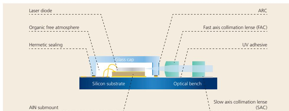
Figure 1: Schematic cross section of a miniaturized WLP laser module with an optical bench
