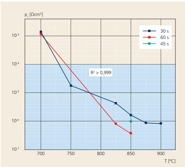
Figure 4: Contact resistance vs. temperature for an annealing time of 30 sec, 45 sec and 60 sec between metal and n-type GaN
