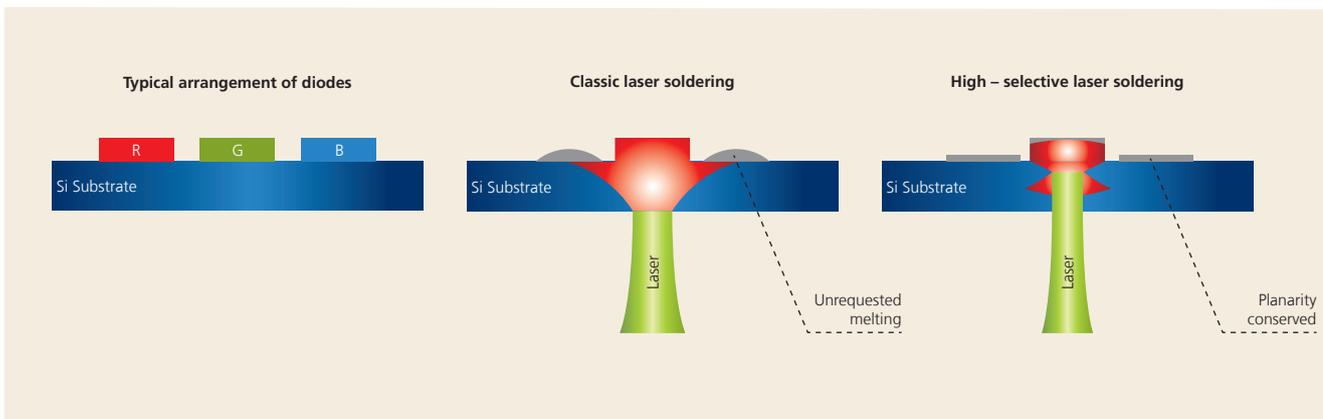
Figure 6: Concept of in-situ laser soldering with direct heat transfer to the soldering pad of a laser diode to further reduce the placement pitch by reduced heat spreading
