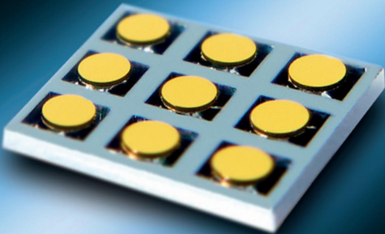
*Figure 1: Array of nine piezoelectric, quasi-static MEMS mirrors with gold reflector*
