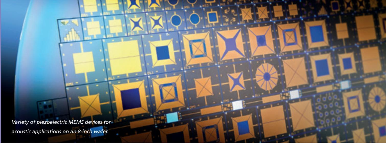
Variety of piezoelectric MEMS devices for acoustic applications on an 8-inch wafer
