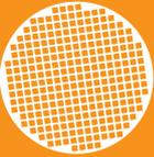
*Figure 3: After the tempering process, the silicon spheres are firmly connected to the silicon wafer by a glass layer (left). In the grinding process they are successively ground off - here (right) the wafer was removed for testing in the middle of the grinding process*
