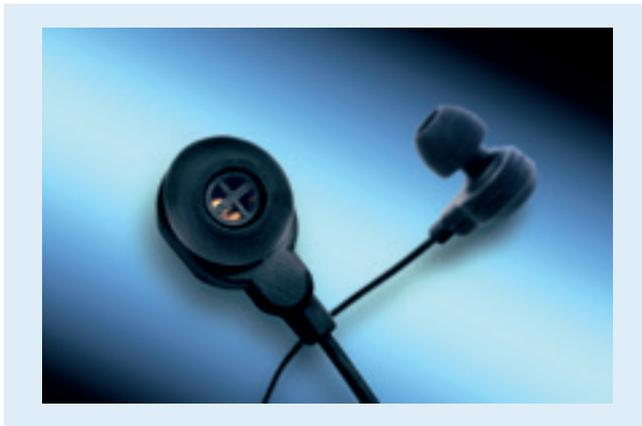
Figure 2: MEMS microspeaker in an in-ear headphone prototype
