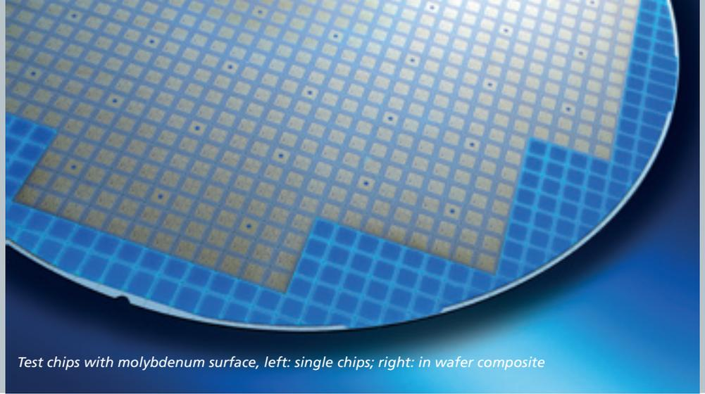
*Test chips with molybdenum surface, left: single chips; right: in wafer composite*
