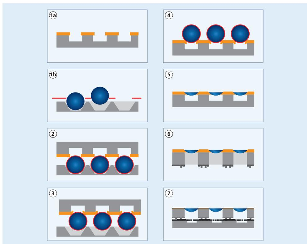
Figure 2: Process flow to integrate Si lenses on the wafer level
