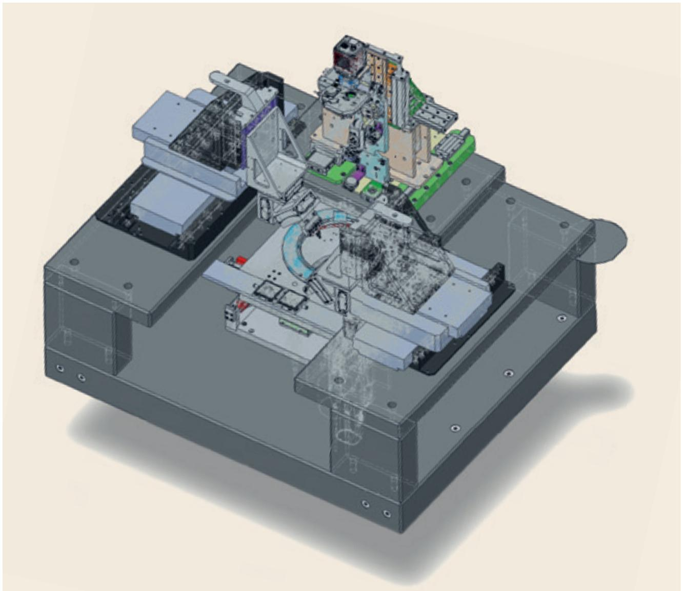
*Figure 5: CAD construction overview on functional modules in the design process of a new ultra-precision assembly station with integrated in-situ laser soldering and active alignment functionality*
