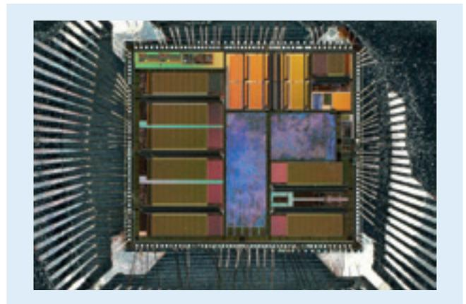
Figure 3: Wet-etch opened chip package
