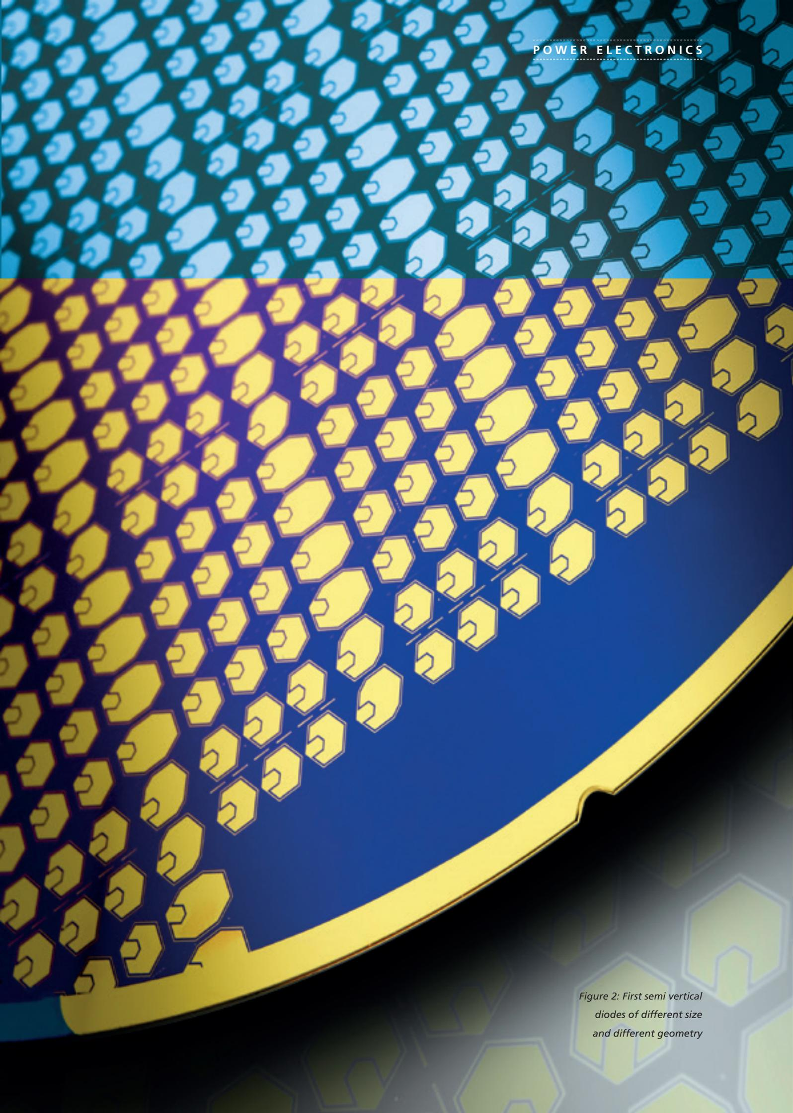
*Figure 2: First semi vertical diodes of different size and different geometry*
