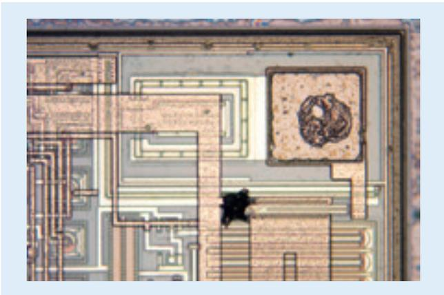
Figure 4: Electrical breakdown between conductive layers on chip
