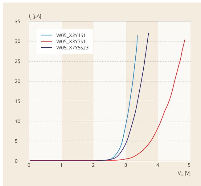
Figure 6: Threshold voltage ( $V_{th}$ ) of semi-vertical GaN devices of different size and different geometry
