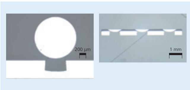
*Figure 4: Cross sections (left) of the Si sphere after bonding to the structured glass / Si wafer and after grinding down the sphere to give a plano-convex form (right)*
