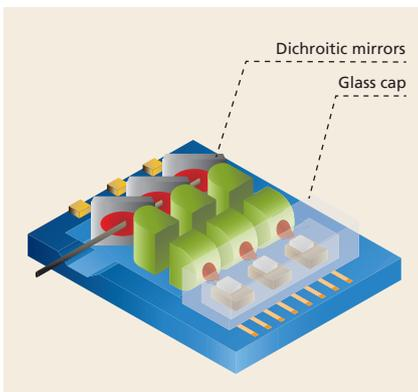
Figure 2: Schematic overview of a first generation multi-color construction of a miniaturized laser module with lateral emission window
