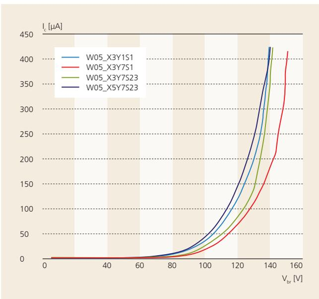
Figure 5: Breakdown voltage ( $V_{br}$ ) of semi-vertical GaN devices of different size and different geometry
