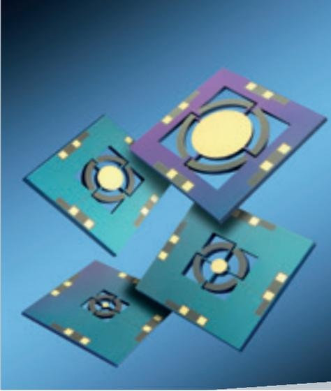
*Different types of piezoelectric micromirrors*
