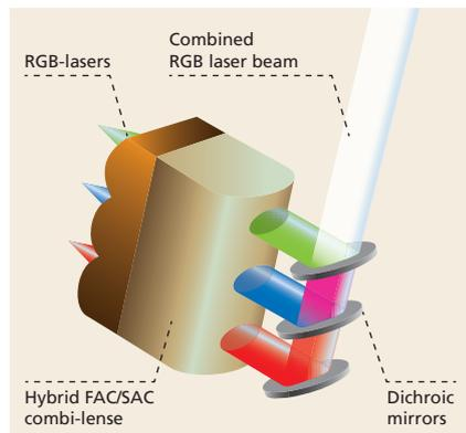
Figure 3: ZEMAX simulation of a hybrid lens design for second generation multi-color laser light engines
