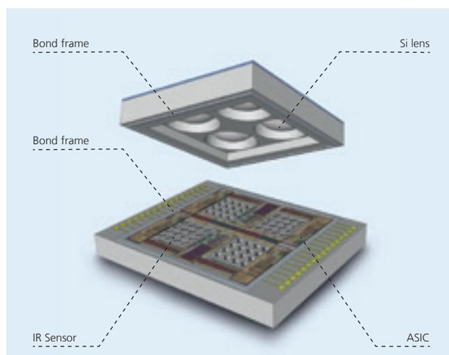
*Figure 1: A typical set-up of wafer level packaged IR sensor, read-out circuit and lens as part of a hermetically tight vacuum package*
