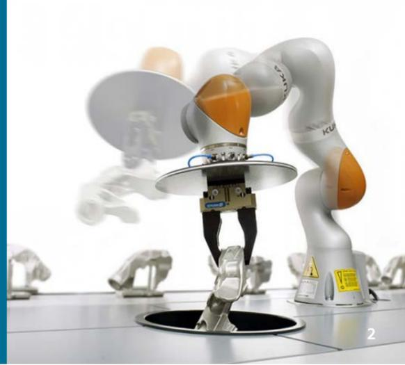
2 The centerpiece of “HeiDetect Inline CT Compact R” at work: An industrial robot lifts a component from the production line and places it in the completely radiation shielded box for testing.
