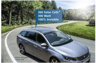
The MorphoColor® glass coating makes it possible to match the solar module's color to that of the vehicle. © Fraunhofer ISE
