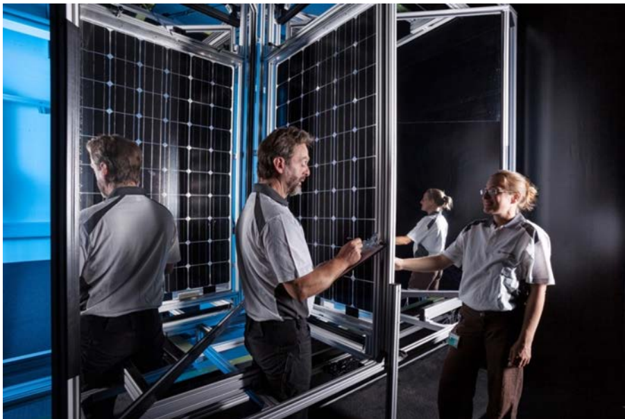
Employees of CallLab PV Modules use a self-developed solar simulator to measure a bifacial module that generates electricity on both the front and rear surfaces. © Fraunhofer ISE
