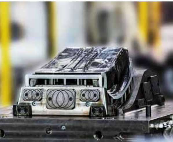
Hybrid seat back made of basalt fiber.
