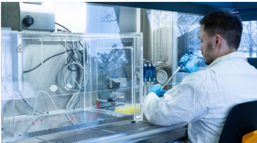
Setup of the aerosolization chamber for the defined investigation of airborne bacterial and viral pathogens up to safety level 2. Additional devices can be integrated for targeted investigations such as the disinfection efficiency of UV-C radiation for airborne pathogens.
