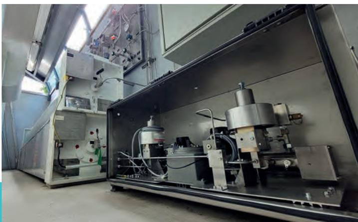
*Hydrogen quality sensor (right) connected to a 900 bar high-pressure tank of the hydrogen refueling station (left).*
