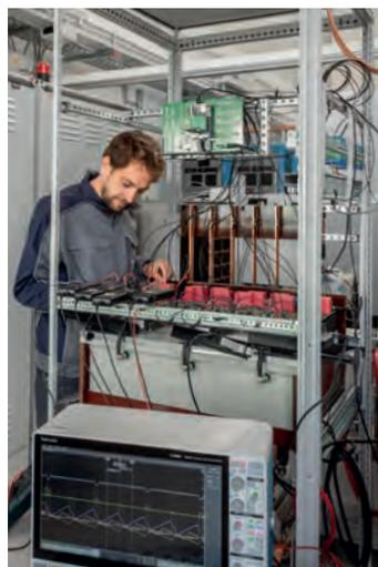
*Design and testbench for SiC inverter stacks in the laboratories of Fraunhofer ISE.*
