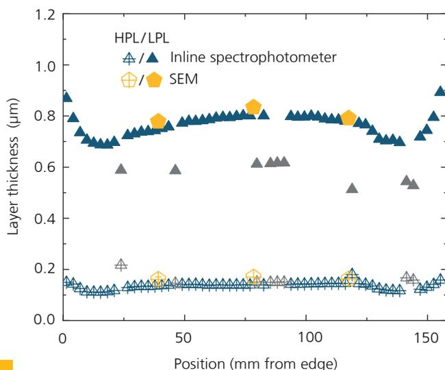
*Thicknesses of the low-porosity and high-porosity layers (LPL and HPL) as a function of the distance from the wafer edge. Gray points represent outliers.*
