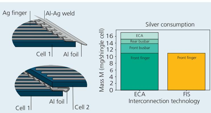
Representation of the FoilMet®-Interconnect shingling (FIS) cell connection (left); silver consumption of a shingle solar cell for two different connection technologies, ECA (electrically conductive adhesive) and FIS (right).
