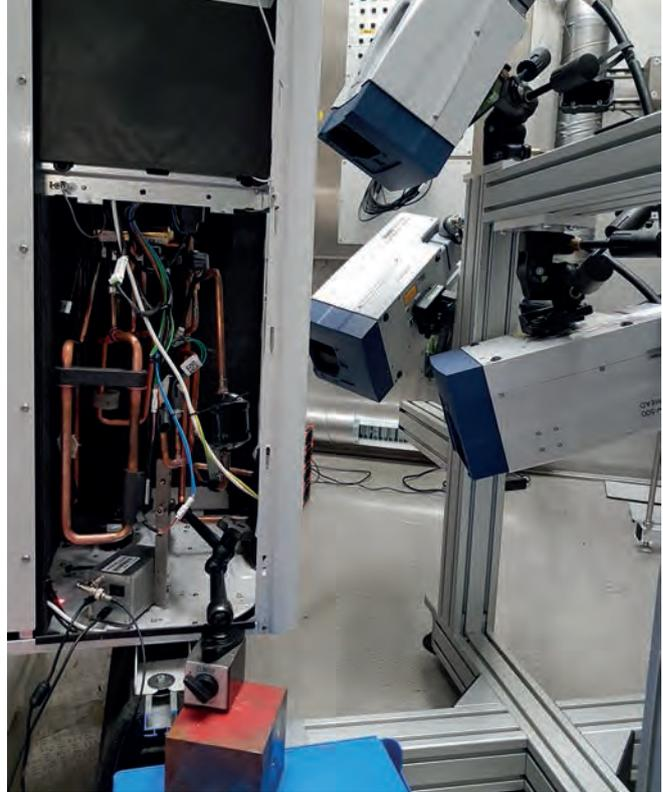
*Structural dynamics investigation of a heat pump with its compressor removed.*
