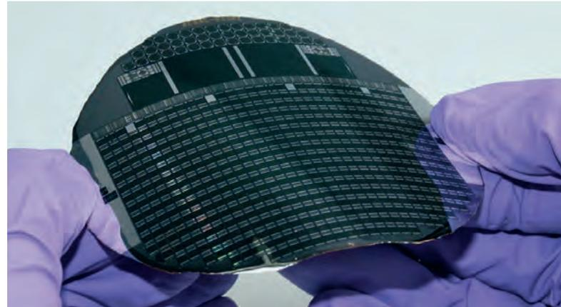
*Flexible 4" wafer with GaAs-based photonic power converters processed as thin-film technology.*
