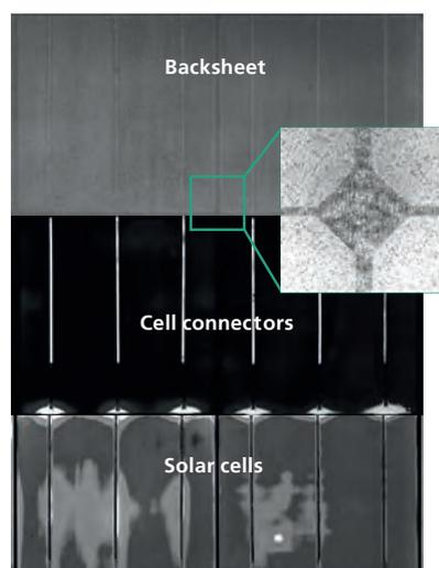
*Scanning acoustic microscope image of different module layers. Inset: Internal cracks in the backsheet.*
