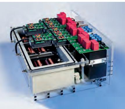
*A 250 kVA inverter stack with 3.3 kV SiC transistors developed at Fraunhofer ISE.*
