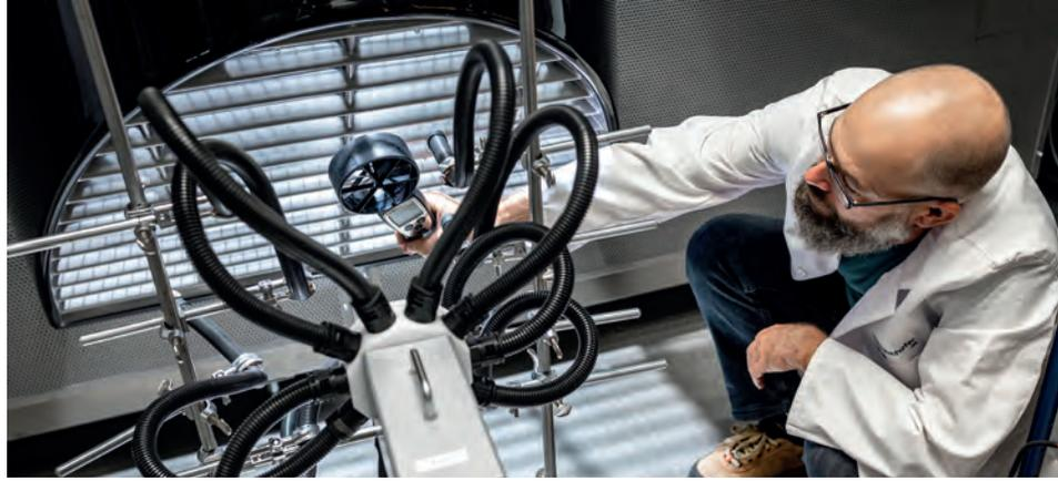
*Measurement of the air temperature and humidity at the outlet of a heat pump installed outdoors.*
