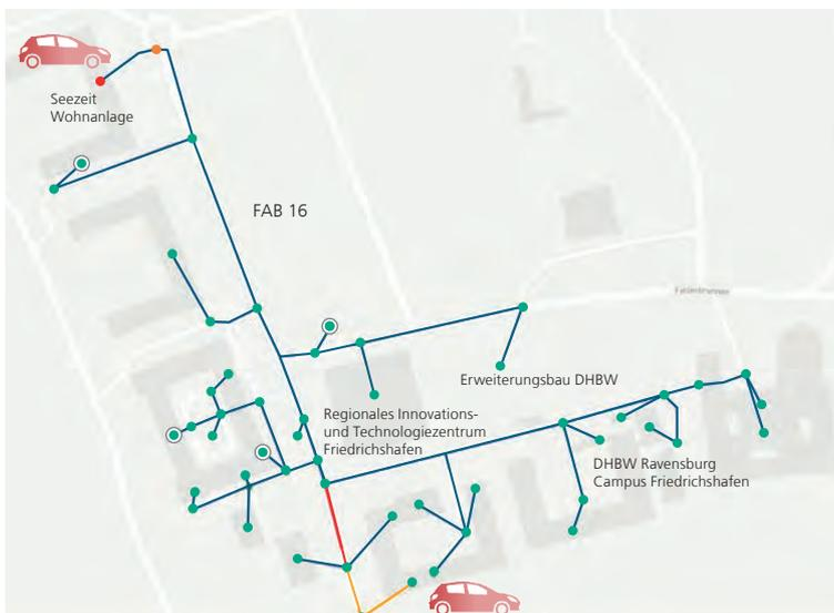
*Visualization of the grid state in an example of a distribution grid with newly connected electric vehicles, which are detected by state estimation.*
