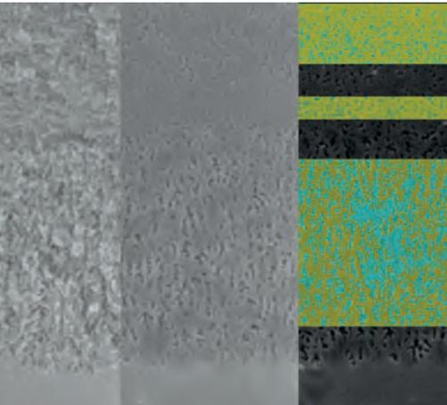
*Cross-section of porous Si layer stack: simply broken (left), infiltrated and ground (middle) and with automatic visualization of porous areas (right).*
