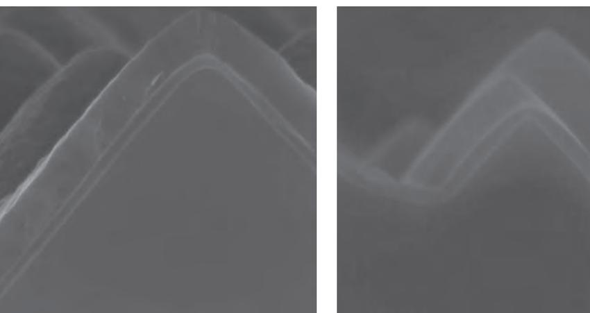
*Scanning electron microscope image of a cross-section of the solar cell front surface, before removal of the TOPCon layer by ADE (left) and afterwards (right).*
