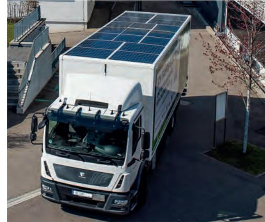
The power electronic integration of the PV modules and thus the connection to the vehicle battery is particularly critical due to the high voltage of > 300 V on the PV side. A specific development within the project, which has been registered for a patent made it possible to meet the safety requirements for road transport and for PV systems and connect the modules directly to the high-voltage system in the vehicle.
