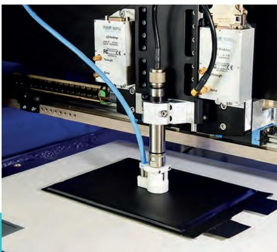
*Non-destructive battery cell characterization using ultrasonic waves.*
