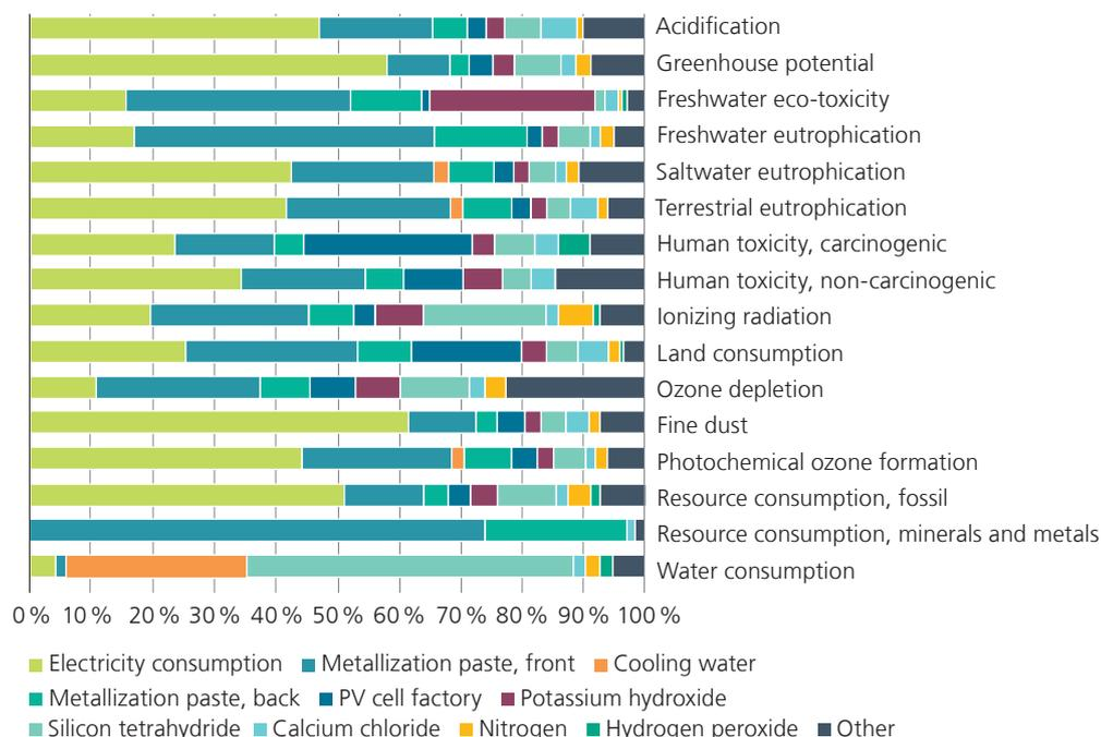
Hotspot analysis according to impact categories related to 1 m<sup>2</sup> of solar cells produced in China. Normalization methodology according to the “Environmental Footprint 3.0” methodology.
