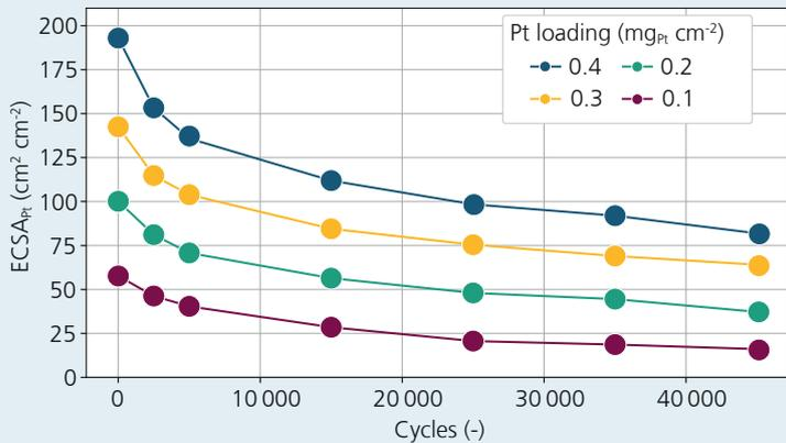
Change in ECSA over 45 000 potential cycles between 0.6 V and 0.95 V for different platinum loadings.
