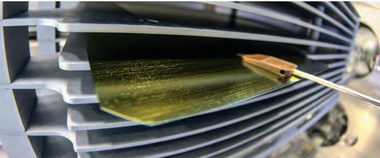
Preparation for TOPCon deposition in a PECVD facility.
