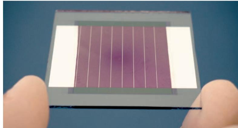
*Mini-module with an area of 9 cm<sup>2</sup> made of organic solar cells that achieves a certified efficiency of 13.94 %.*
