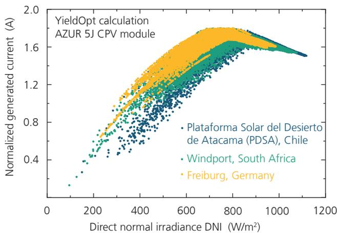
*Generated current of a CPV module normalized to the irradiance DNI of 1000 W/m<sup>2</sup> in different locations (Chile, South Africa and Germany).*
