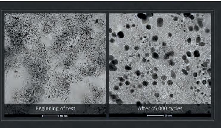
TEM images of Pt nanoparticles in a non-degraded cathode (left) and a cathode that has degraded during 45 000 potential cycles (right).
