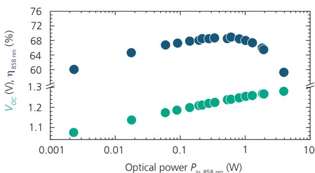
*The measured performance parameters, the monochromatic efficiency  $\eta_{858\text{nm}}$  and the open circuit voltage  $V_{OC}$  of the GaAs-based record cell with an area of 0.054  $\text{cm}^2$ , plotted as a function of the optical power at a wavelength of 858 nm.*
